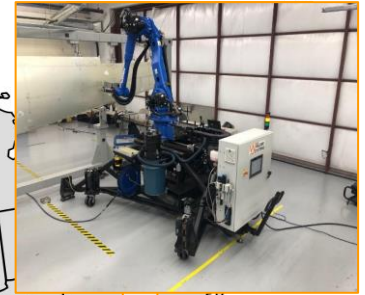
M600 Wing Drilling Vero Beach, FL
